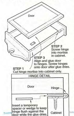
Recently, I made a clock with a door that required mortising hinges into the case, but not the door. However, I had difficulty figuring out how to precisely position the hinge on the door to drive the screws. Finally, it occurred to me to glue the door to the hinge until I could permanently attach it.
